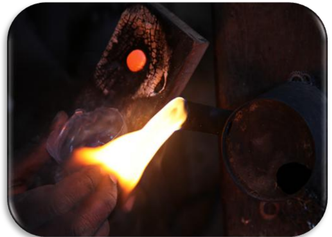
A torch with a hot flame is used to melt the silver. We decide the silver will be shaped into a decorative turtle.
